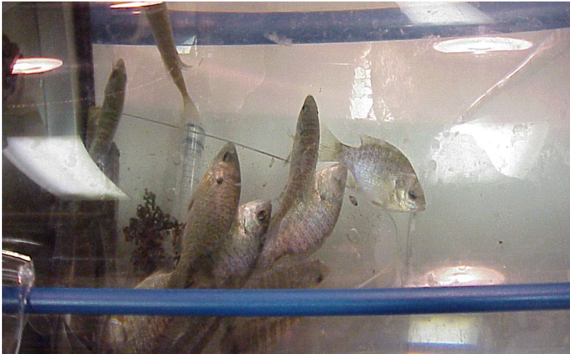
Figure 4.13. Bluegill Reacting to Pressure Spike During Turbine Passage Sequence
