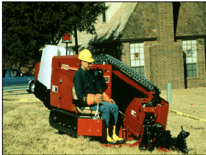
Figure 1. Typical HDD Rig for Gas Applications
