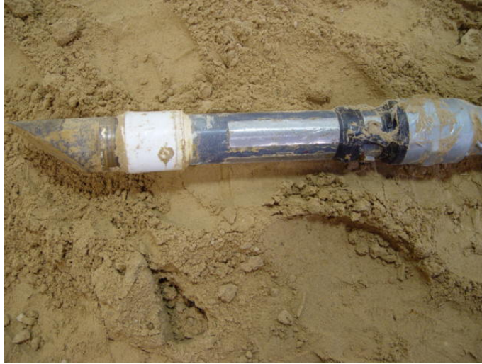
Figure 4b. Close-up of prototype with steel shim sense elements
