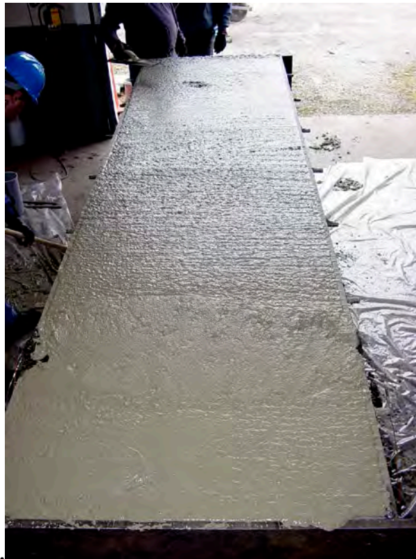
Fig. 10. WesDyne concrete specimen after all concrete poured [2]
