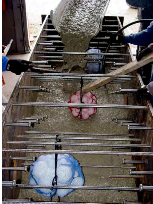
Fig. 9. WesDyne 3X3X10 Specimens showing void simulators [2]
