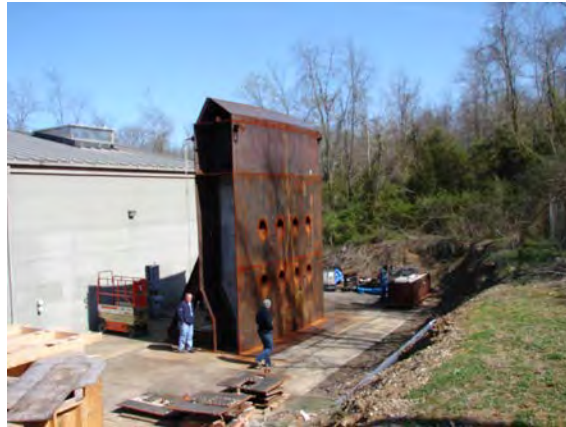
Fig. 11. WesDyne Westinghouse AP1000 Shield Building NDE Evaluation Section [2]
