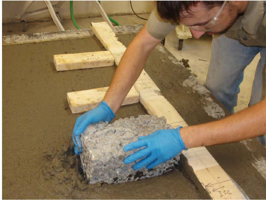
Fig. 21. Installing the surface level pervious concrete prism and two short boards holding the triangular plates used to make the simulated cracks [8]
