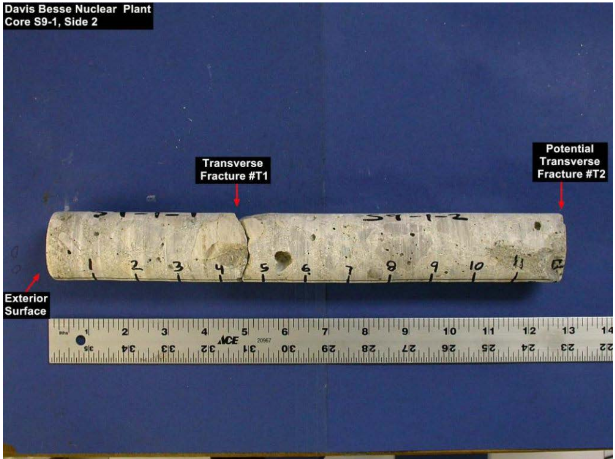
Fig. 7. Laminar Cracking at a core location [42]
