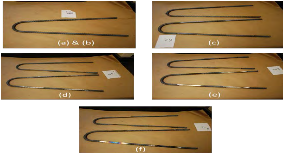
Fig. 16. Different levels of simulated corroded U-shaped rebar
