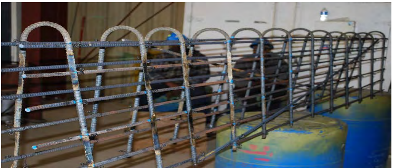
Fig. 17. F-shaped bolt-down barrier fabrication with simulated corrosion
