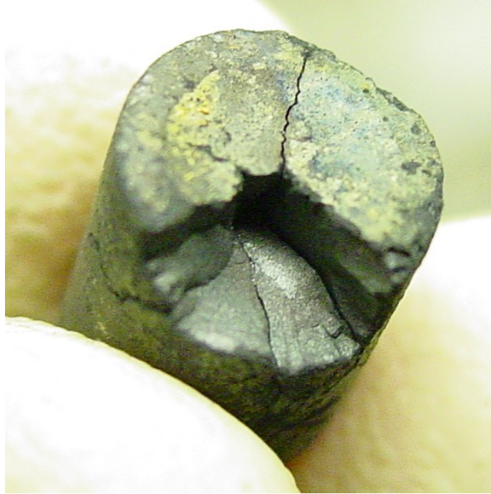
Figure 8 Cracks in pellets heated with an electric heat gun and then thermally quenched
