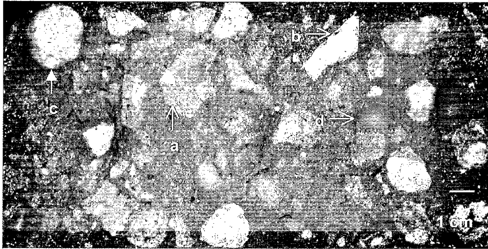
Figure 9. Fracture Surface of 50 BFS Concrete with Recycled Concrete Aggregate Showing Examples of: (a) Fractured Old Mortar; (b) Fractured Stone; (c) Unfractured Stone and (d) Stone Pullout.
