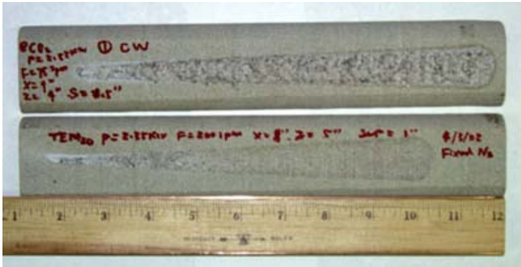
Figure 4. Comparison of linear tracks produced with changed (top) and fixed (bottom) purging gas position. Fixed gas nozzle helped to produce a clean track.
