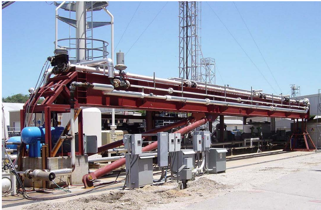
Fig. 2.1 Mast together with the hydraulic cylinders
