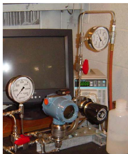
Fig. 3.4 Air and liquid injection systems
