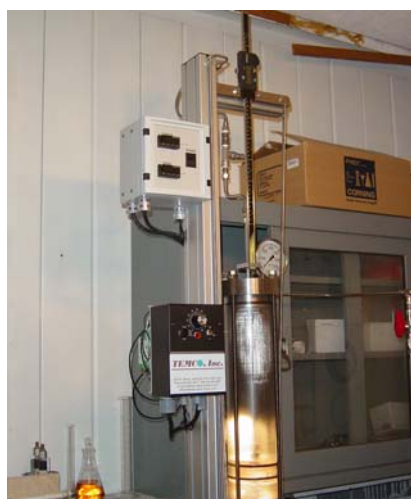
Fig. 3.3 Foam generator cylinder
