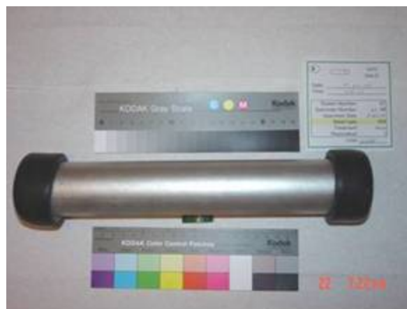
Figure 20. Welded tube, sample 57D20 (Type 304).
