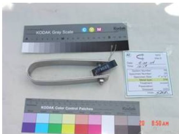
Figure 29. U-bend coupon, sample 78D20 (Type 316).
