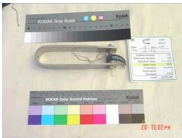
Figure 27. U-bend coupon, sample 73D20 (Type 304).
