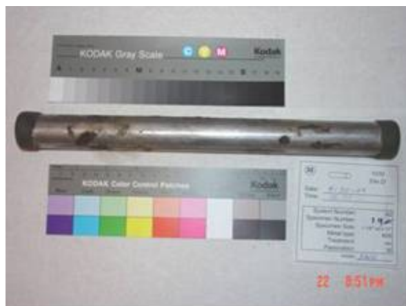
Figure 21. Welded tube, sample 62D19 (Type 409).
