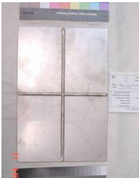
Figure 15. Front side cross-welded plate, sample 54D19 (Type 301).
