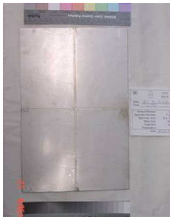
Figure 16. Backside cross-welded plate, sample 54D19 (Type 301).
