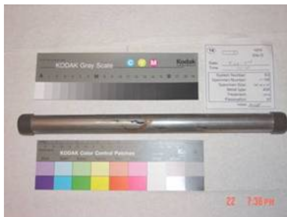
Figure 24. Welded tube, sample 63D20 (Type 409).
