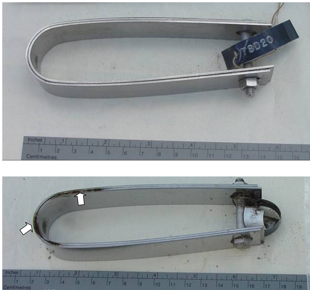
Figure A.1. Double U-bend samples, Type 316, Sample 78D20 (top) and Type 434, Sample 81D20 (bottom). Note crevice corrosion (arrows) in Type 434 sample.
