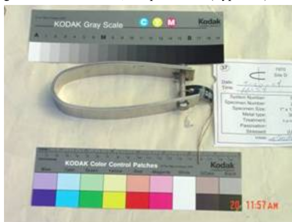
Figure 26. U-bend coupon, sample 71D20 (Type 301).
