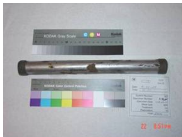
Figure 23. Welded tube, sample 63D19 (Type 409).
