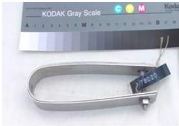
Figure 13. Stressed U-bend coupon.
