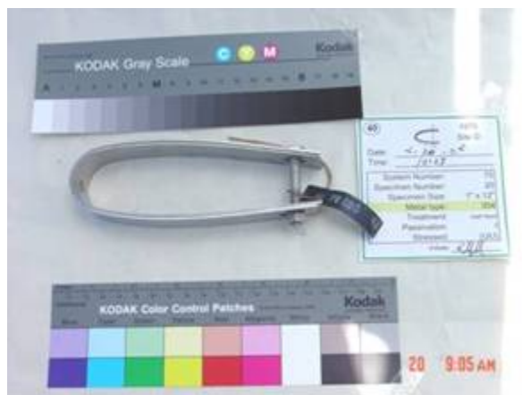
Figure 28. U-bend coupon, sample 75D20 (Type 304).
