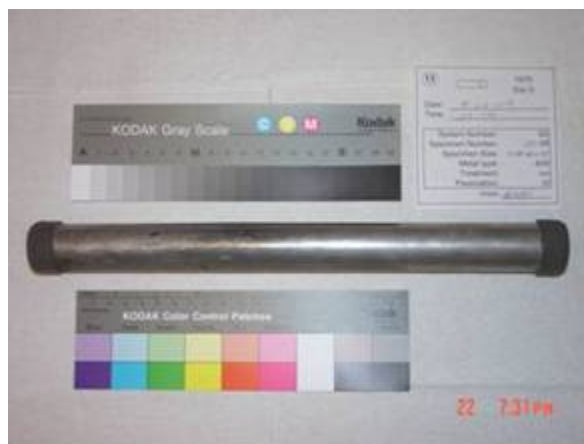
Figure 22. Welded tube, sample 62D20 (Type 409).
