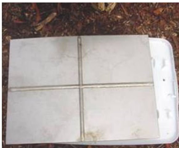
Figure 12. Cross-bead welded plate after retrieval.
