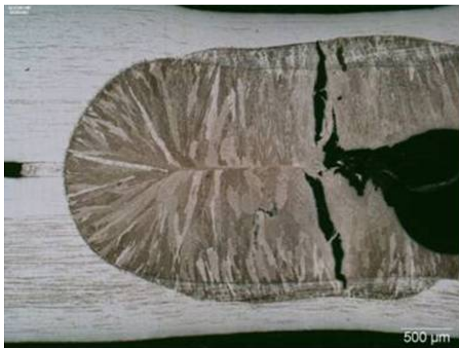
Figure 44. System 78 (Type 316) 25X photograph of cross section with large shrinkage voids. No corrosion visible.
