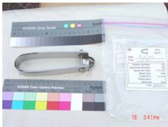
Figure 30. U-bend coupon, sample 81D20 (Type 434).
