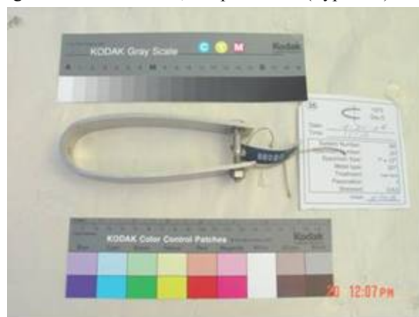
Figure 25. U-bend coupon, sample 68D20 (Type 301).
