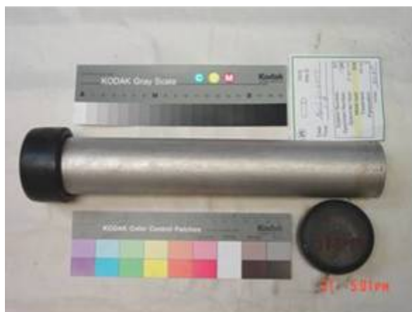
Figure 19. Welded tube, sample 57D19 (Type 304).
