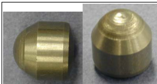
Figure 38. Two Views of the Round Top Drill Bit Insert. The insert is typical of the cutting tools placed on rotary drill bits. (Orientation of the fibrous monolith was right to left, from the round top to the flat base.)
