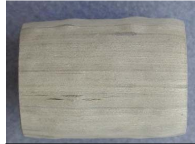
Figure 14. Cracking, delaminations, and bloating resulting from binder burnout and sintering.
