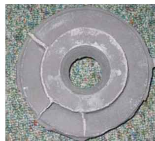
Figure 57. Rib defects on disc cutter
