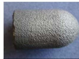
Figure 33. FM insert after container-less HIPping
