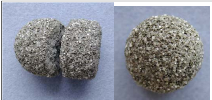
Figure 31. . FM Insert after binder burnout and sintering in container confinement with coarse sand
