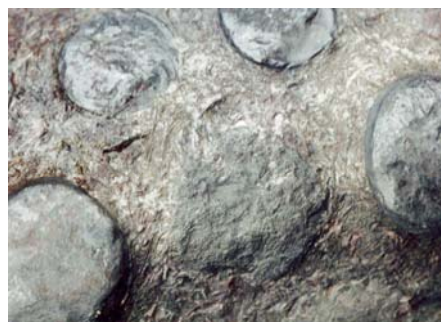
Figure 42. Highly Worn FM Insert on a Worn Superior Rock Bit Drill Bit. Compare the worn insert (center) to the surrounding current art inserts. The two current art inserts at the top exhibit brittle failures.
