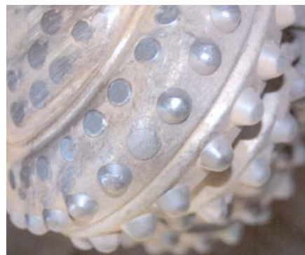
Figure 41. Current Art and Fibrous Monolith Inserts on a Worn Superior Rock Bit. The FM insert in the center has worn more than the current art inserts, although no brittle failures have occurred like the small chip on the insert to the left of the test insert.
