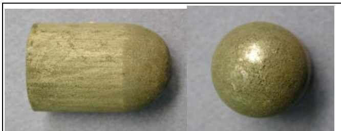
Figure 32. . FM Insert after binder burnout and sintering in container confinement with finer sand
