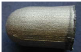
Figure 36. FM insert after sintering and low pressure HIPping
