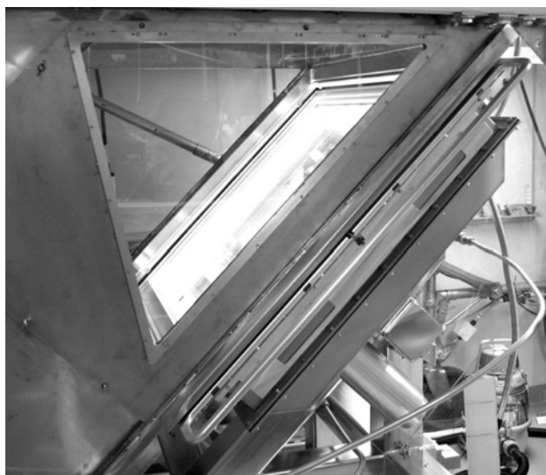
Figure 9: Photograph of an illuminated LM5 mirror taken through the viewing window in the side of the elbow enclosure.
