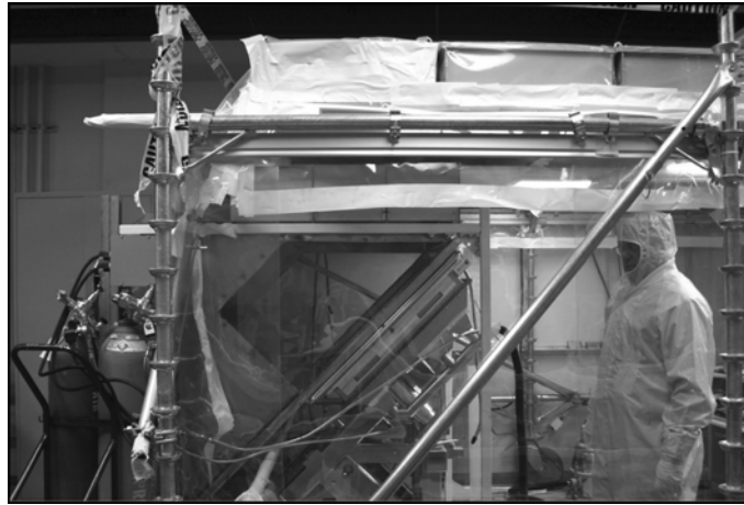
Figure 15: Experimental elbow with prototype viewing and debris removal systems in a clean room.
