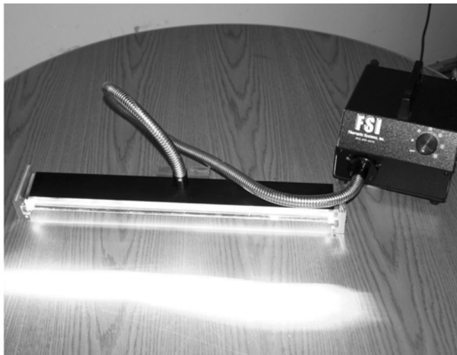
Figure 8: Fiber optic bar light used to illuminate the mirror surfaces.
