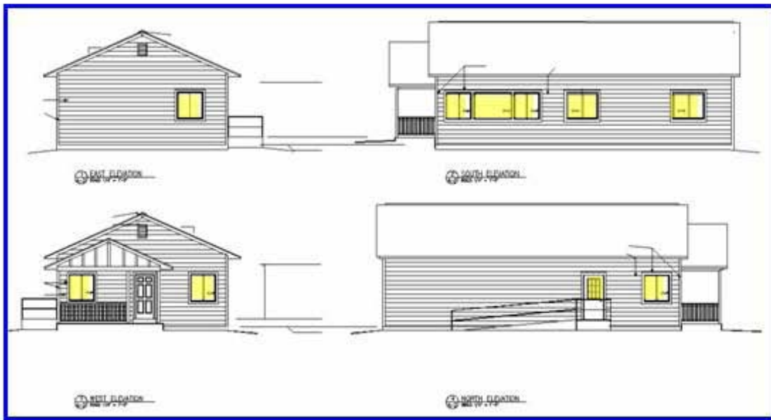
Figure 5. Window distribution for sun tempering in the ZEH
