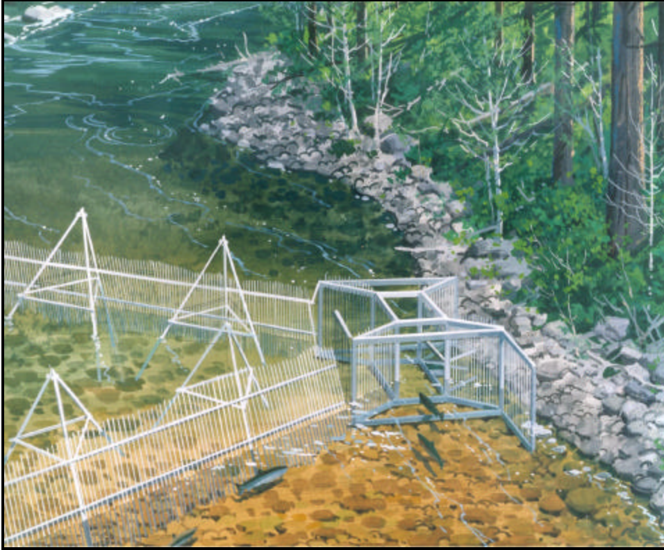
Figure 2. Artist's rendition of the underwater video fish counting station demonstrating the 0.86 by 0.71 m fish passage opening.
