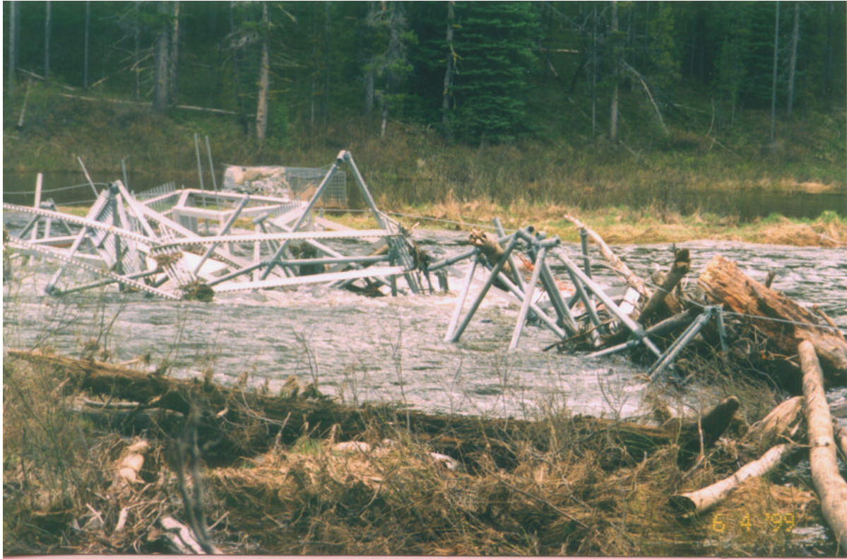
Figure 15. Failed Secesh River fish counting station.
