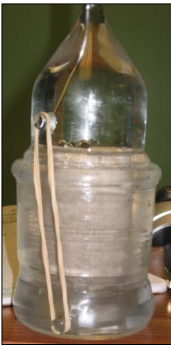
Plate 2 Detail of imbibition cell
