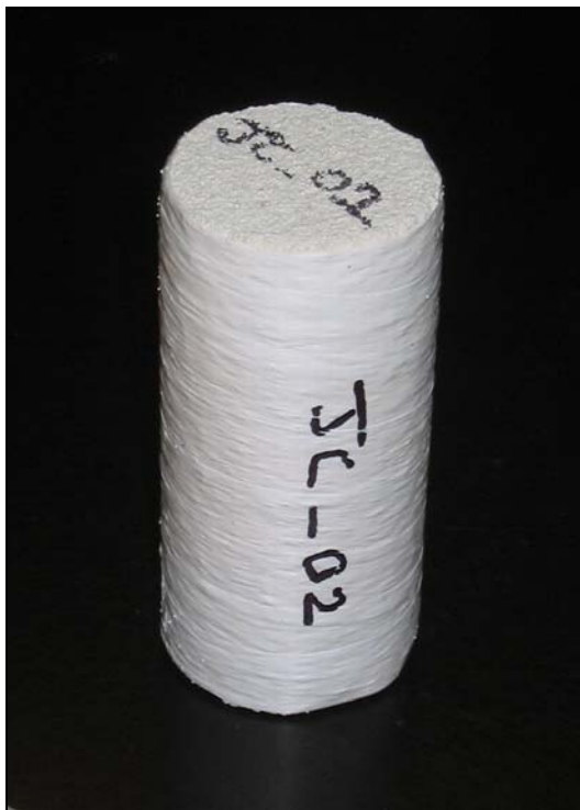
Plate 6 Core material: Joulter Cay oolitic outcrop wrapped in PTFE tape
