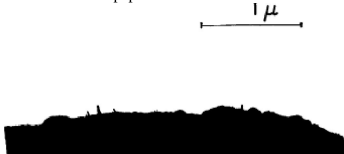
Fig.2.17 Shadow gram of an emitter on a tungsten electrode [14]
