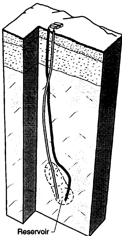
Figure 1. The Phase II HDR reservoir. The reservoir is ellipsoidal in shape with gross dimensions of approximately 200x1000x1000 meters. It is centered about 3.6 kilometers below the surface.
