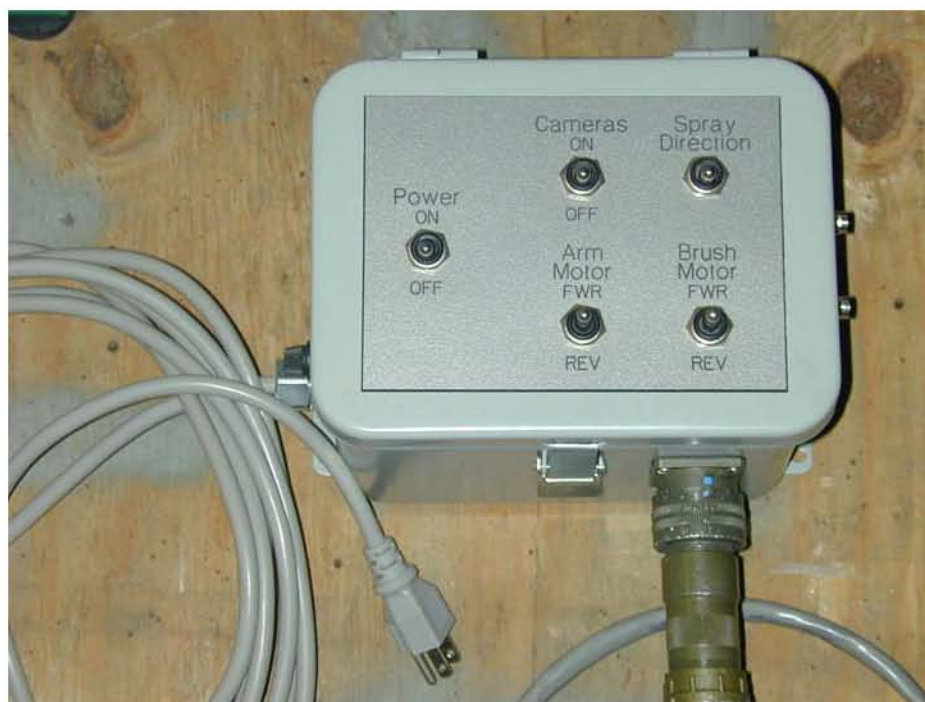
Figure 2-6 External Control Box
