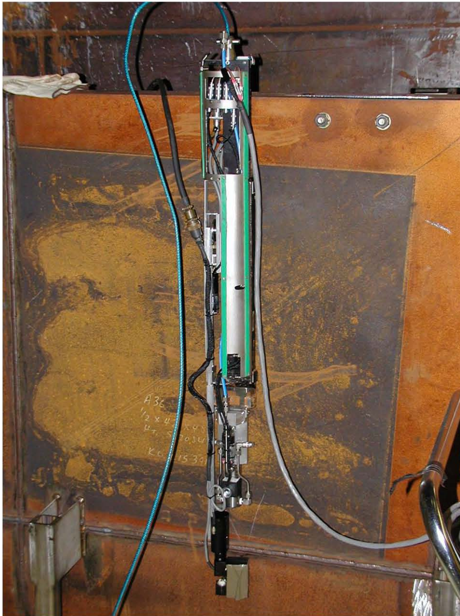
Figure 2-5 Modified Wall Crawler on Tank Mockup Wall
