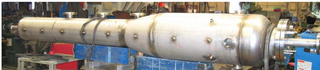
Figure 5.10 Tube bundle condenser secondary pool tank
