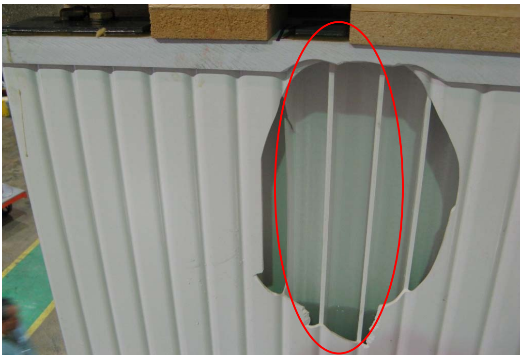
Figure 12: Fracture on the extrusion
