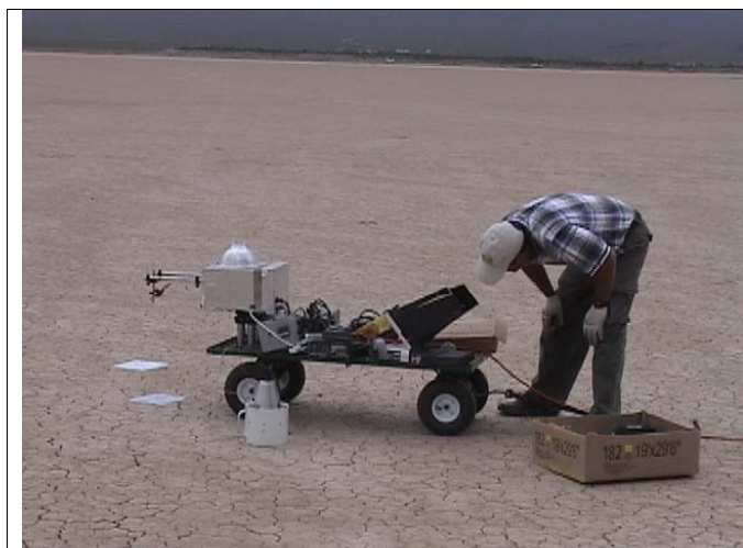
Figure 2 shows preparations made with the mobile Fourier transform infrared spectrometer prior to data collection.
