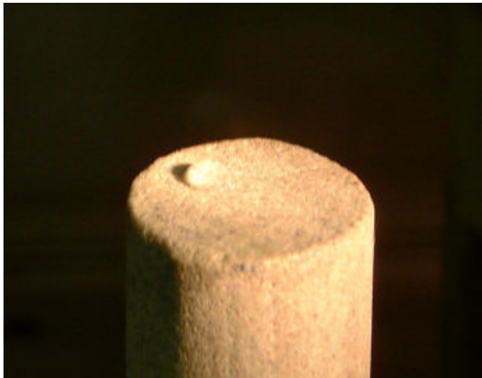
Treated Berea (BB-6); Contact Angle: 60-70 degrees; T=80^{\circ}\text{C}
