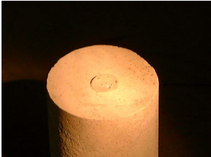
Treated chalk (CC-7) contact angle: 60-65 degrees; T=80^{\circ}\text{C}
