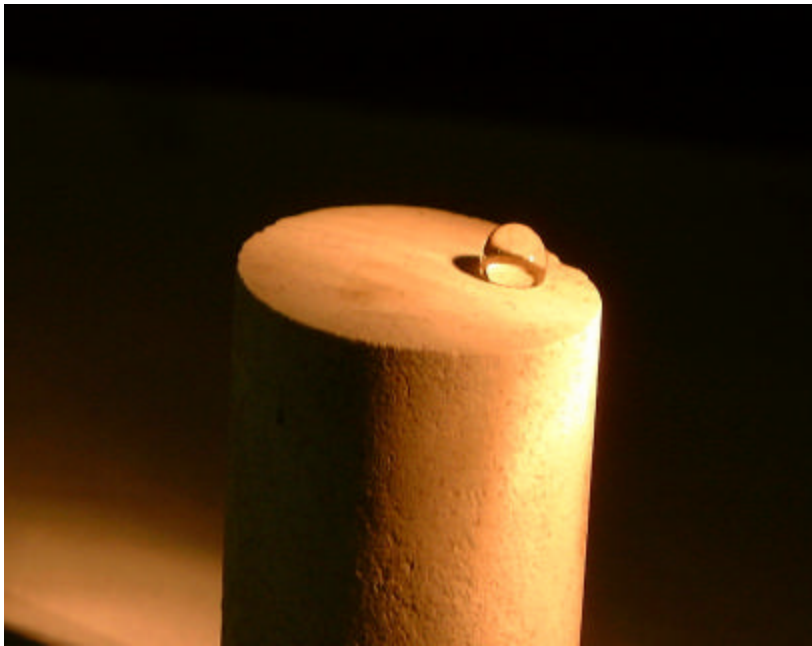
Treated chalk (CC-7); Contact Angle: 110-115 degrees; T=24^{\circ}\text{C}
