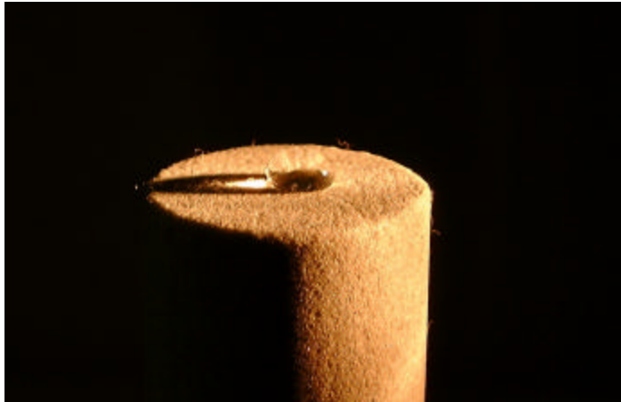
Treated Berea (BB-6); Contact Angle: 120-130 degrees; T=24^{\circ}\text{C}
