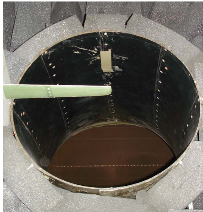
Figure 4b. Blade section immersed in open jet flow.
