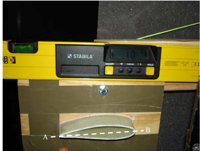
Figure 4a. Angle of attack was measured with an electronic level.
