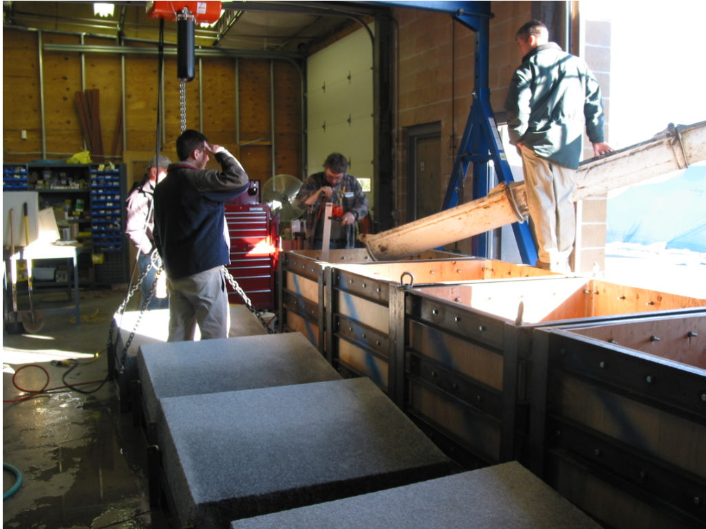
Figure 4: Pouring concrete for first block
