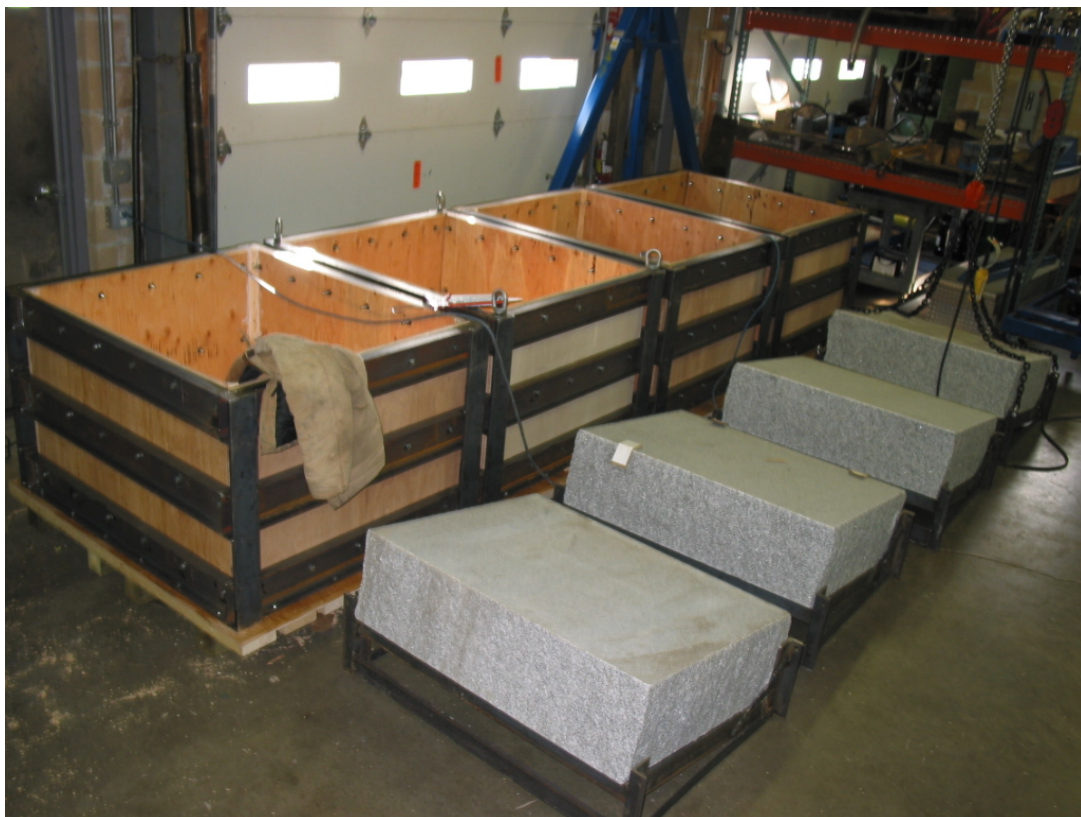
Figure 2: Granite blocks and concrete molds ready for assembly
