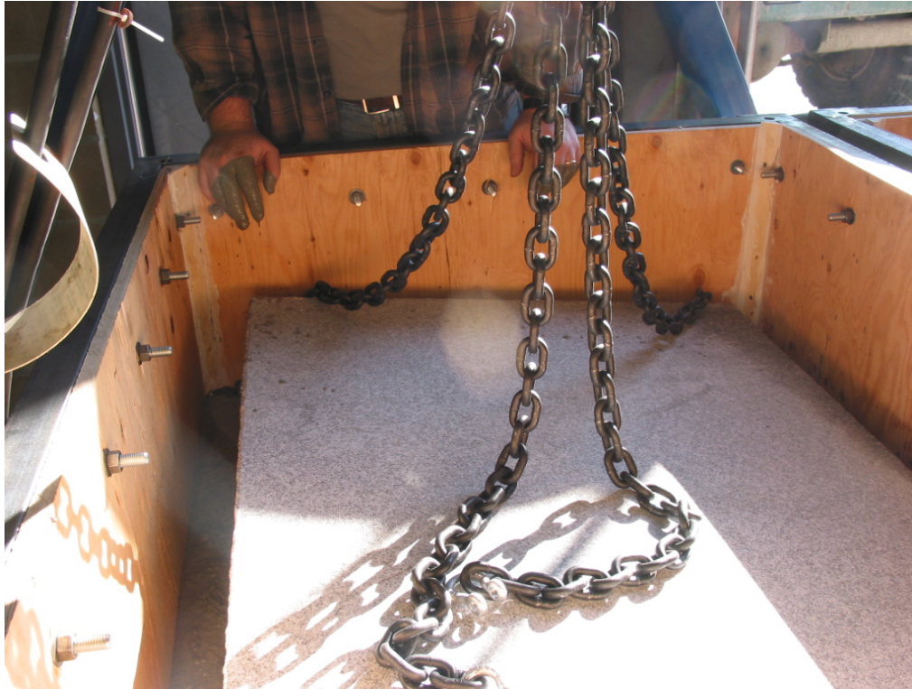
Figure 3: Positioning granite block at 10° angle before concrete pour
