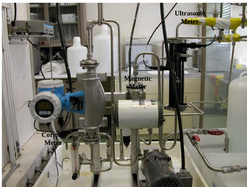
Fig. 6. Close-up view of instruments installed in the uranyl nitrate flow loop. The three instruments (left to right) are as follows: an Endress+Hauser Promass 83F Coriolis flowmeter, a Yokogawa ADMAG AE magnetic flowmeter, and a Controlotron 1010N1 clamp-on ultrasonic flowmeter.
