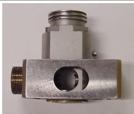
Fig. 1. Weld fixture for confined pinch welds.
