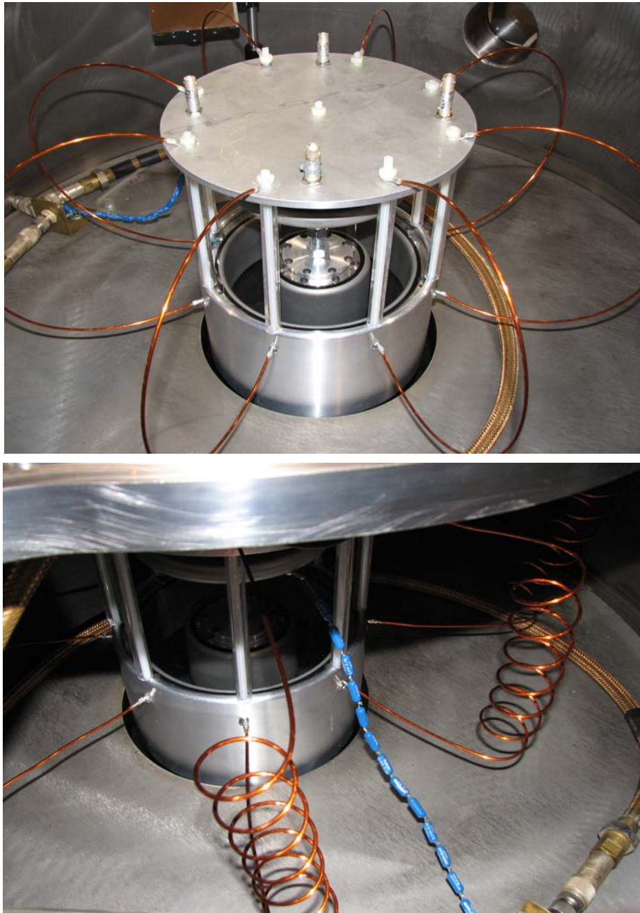
Figure 25. Photos of experimental setups where inductance was added to increase circuit impedance. The top photo shows the 8 x straps setup and the bottom photo shows the 8 x L1 setup.
