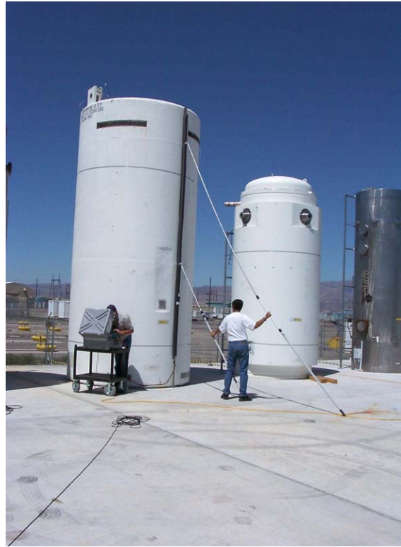
Figure 8. Surface temperature measurements were obtained using a thermocouple rake.
