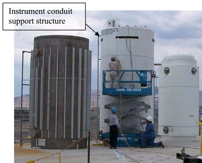
Figure 9. Electrical conduit is visible from behind the VSC-17 cask, which prevented obtaining surface temperature measurements on the west side of the cask.
