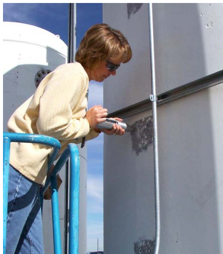
Figure 15. Schmidt rebound hammer testing on the VSC-17 cask.
