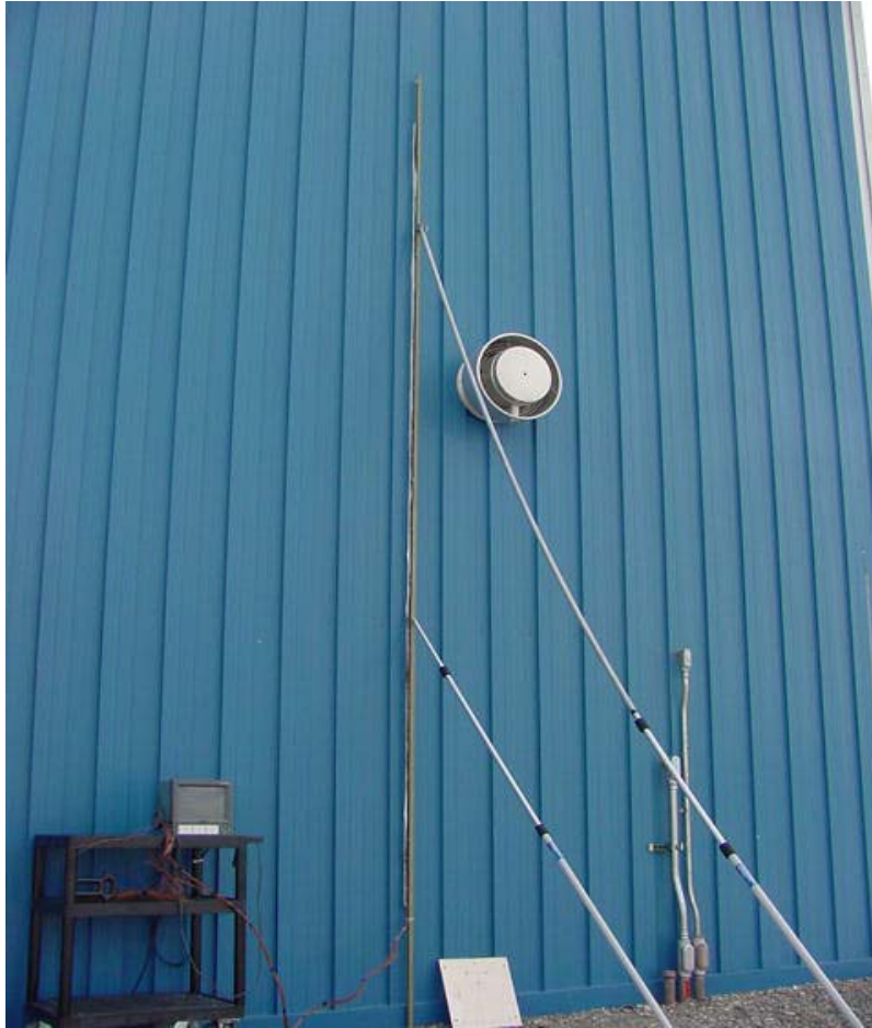
Figure 7. Laboratory building wall test of insulated thermocouple rake.
