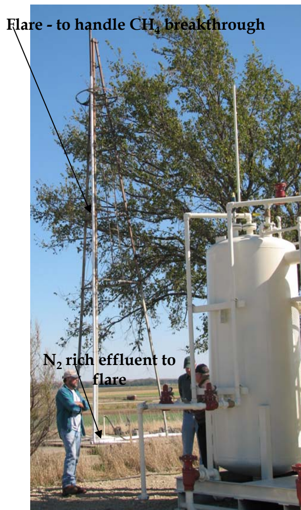
Figure 10: A) Picture showing the vent line connecting to the flare. B) Picture showing the bull nipple and the hopper used to load the towers with activated carbon.
