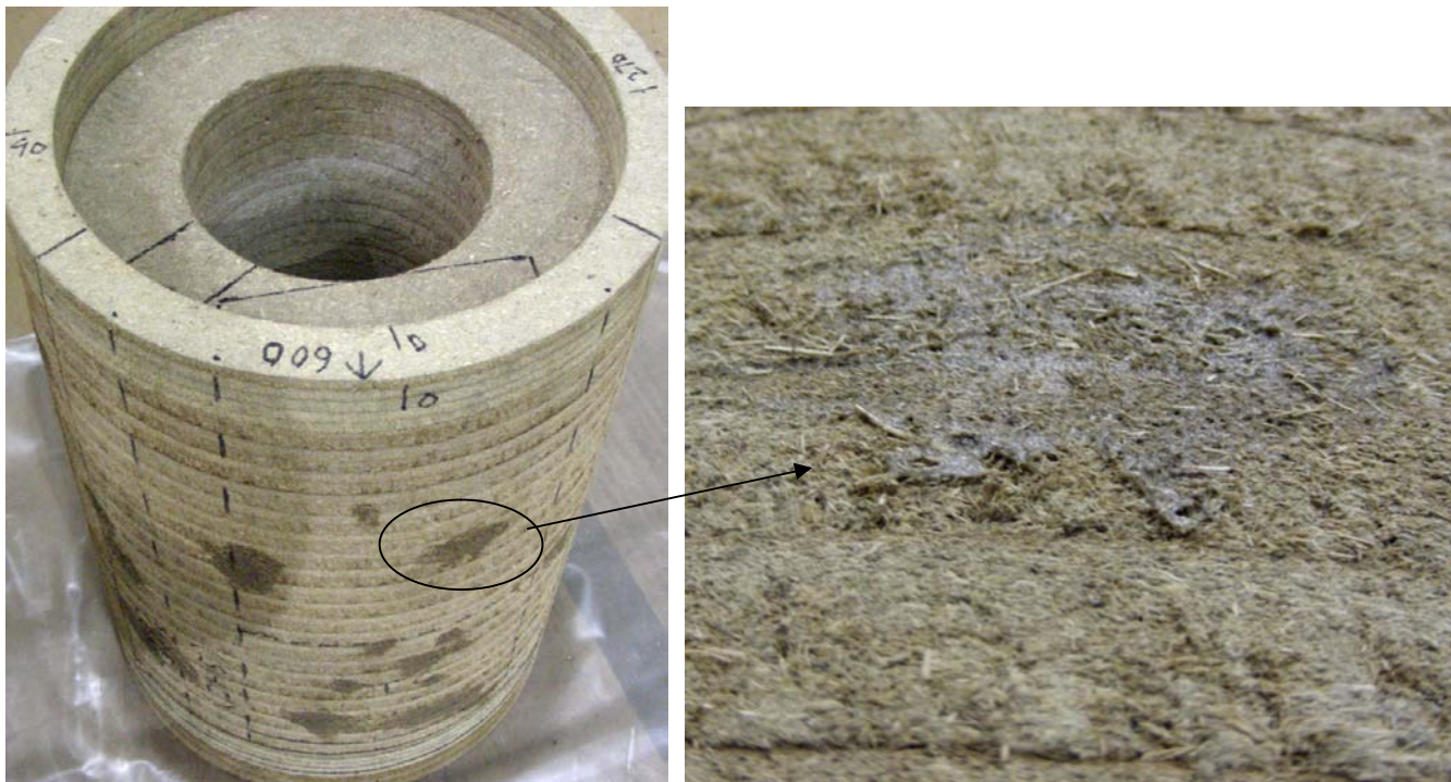
Figure 1. Dark regions on the OD surface of the lower fiberboard assembly
