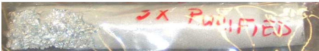
Fig. 4. Zinc sample, after 3 stages of purification.
