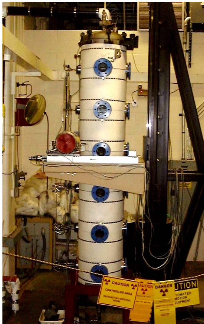
Figure 7. Photograph of the Sandia slurry bubble-column reactor facility. Also shown is the vault for the gamma source mounted on the two-axis automated traverse.
