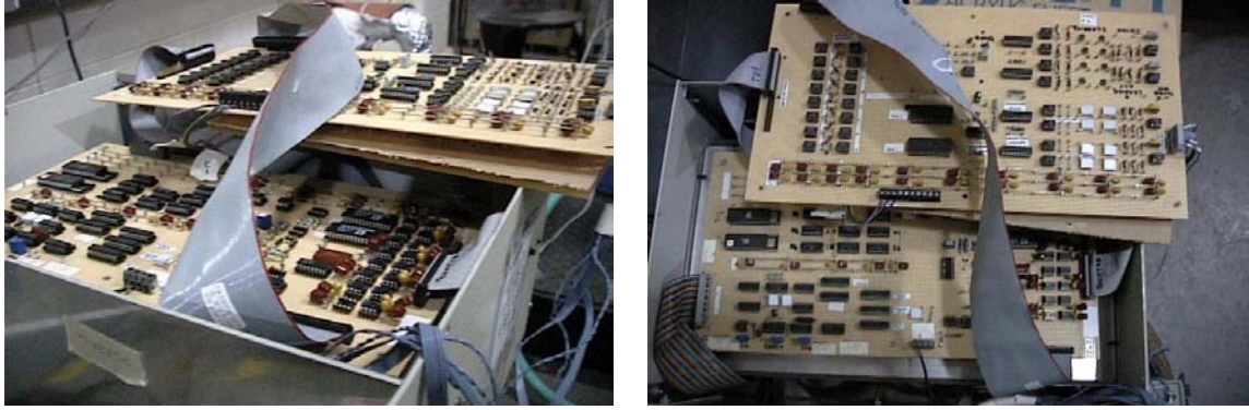
Figure 4. Photographs of the circuits boards inside the EIT electronics box.
