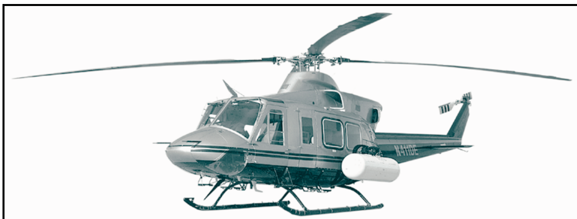
Figure A-1 Bell-412 Helicopter with Detector Pods. The white detector pods, mounted on the sides, each contain six detectors.
