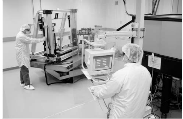
Fig. 1 Photo of an on-line laser conditioning station used to laser condition larger aperture ( up to 40 cm x 80 cm) mirrors and polarizers.
