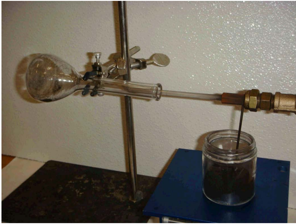
Figure 11. Co-axial delivery of particulate into an enclosed volume (lab flask) using a micro-Venturi to entrain dry powder into the carrier gas (air) flow.
