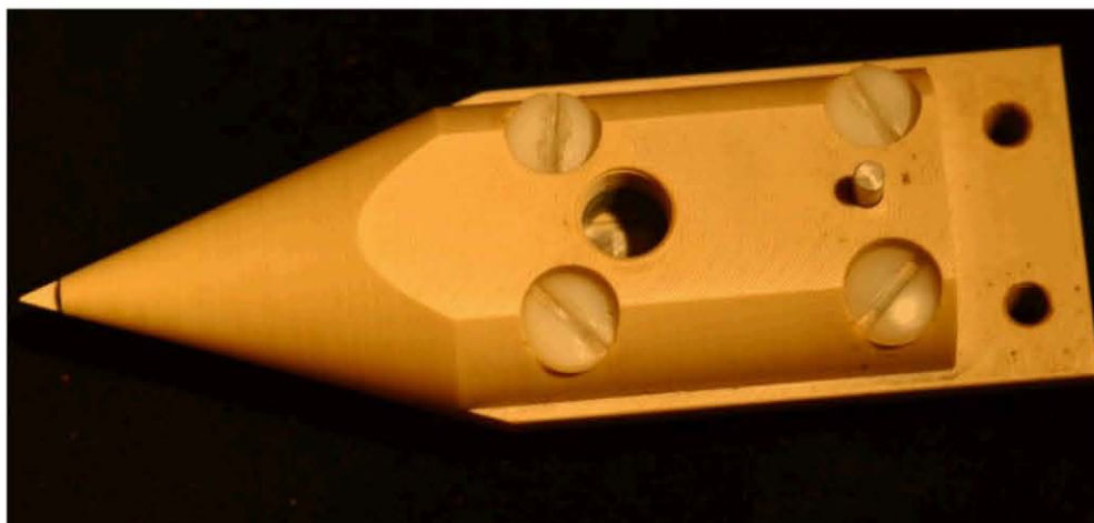
Figure 6. Electrodynamic atomizer used in UC Davis experiments as supplied by Terronics Development, Inc. Liquid flow into atomizer is through the 1/8”NPTF threaded port in the center and high voltage supply is through the stainless steel pin to right of liquid port.
