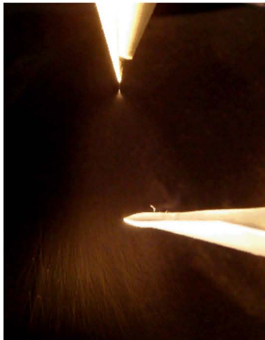
Figure 9. Deflection of spray path caused by grounded spatula placed in proximity of spray.
