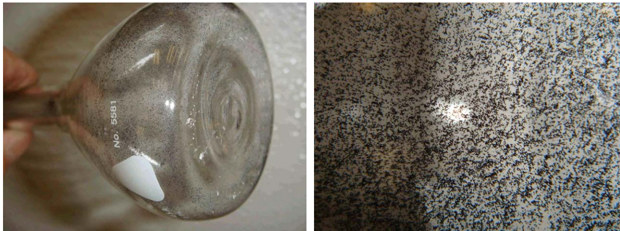
Figure 12. Deposition resulting from gas carrier delivery of particles into an enclosed, relatively difficult to coat surface.
