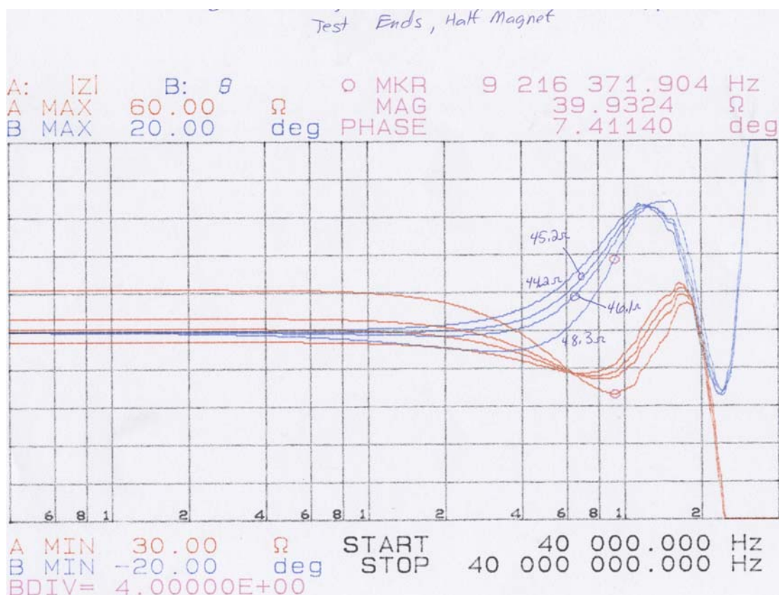
Figure 11, Magnitude and Angle vs. Termination Resistance for C2010 Prototype
