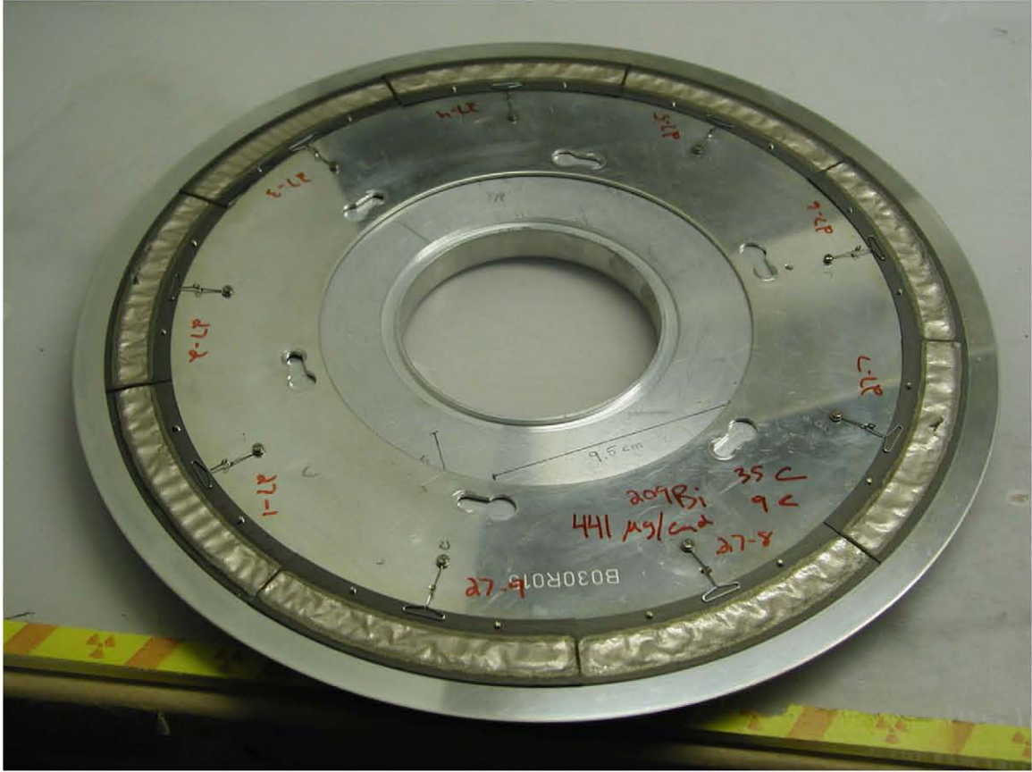
Figure 2.1: ^{209}\text{Bi} target wheel used in experiments with BGS. Individual targets are mounted on the periphery of the wheel, seen as textured strips. Numbers indicate individual target number (e.g.: 27-1) and target set properties.
