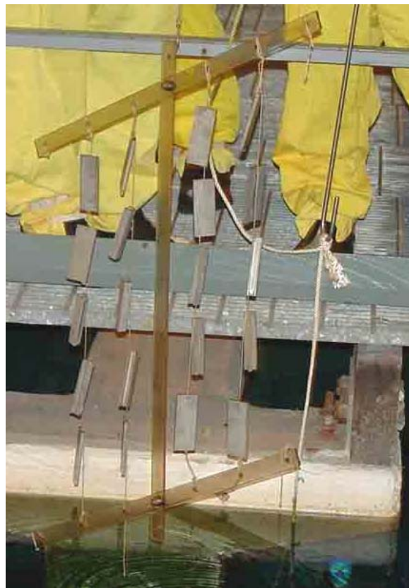
Figure 7. Hanging furniture rack coupons removed from L-Basin.
