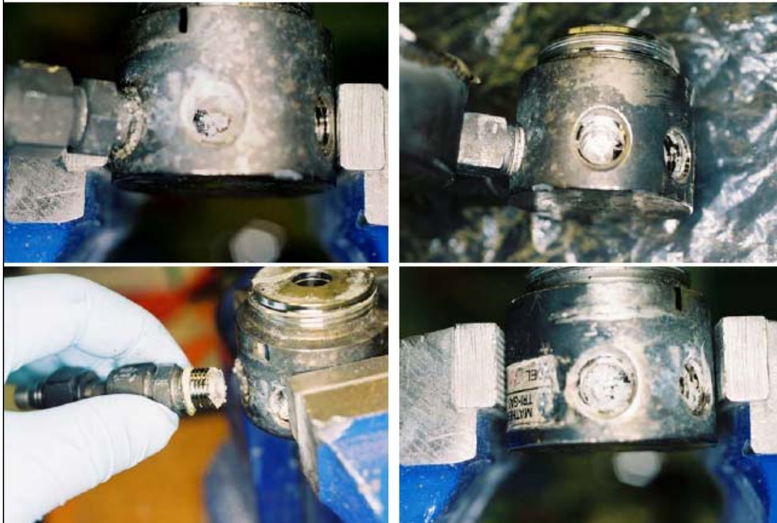
Figure 4. AEC's PCV-23, showing ports after the accident.
