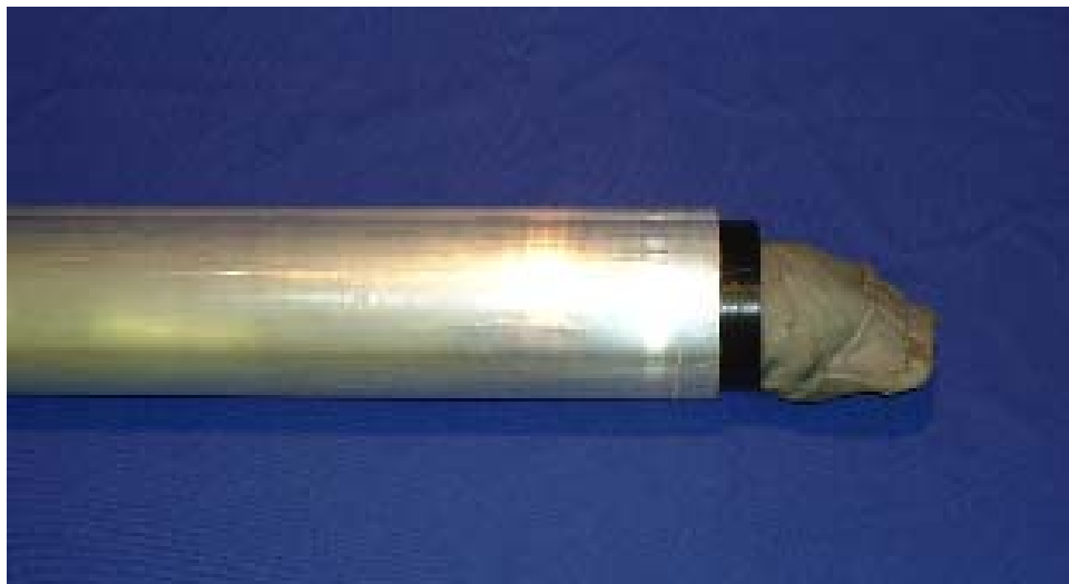
Figure 9 - Silicon Rubber Bag Inserted into Liner
