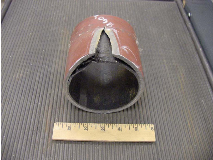
Figure 23 - Section Taken Hydrostatic Test Rupture of Long, Shallow Simulated Corrosion Damage in Pipe Section Containing Fiber-Reinforced Composite Liner
