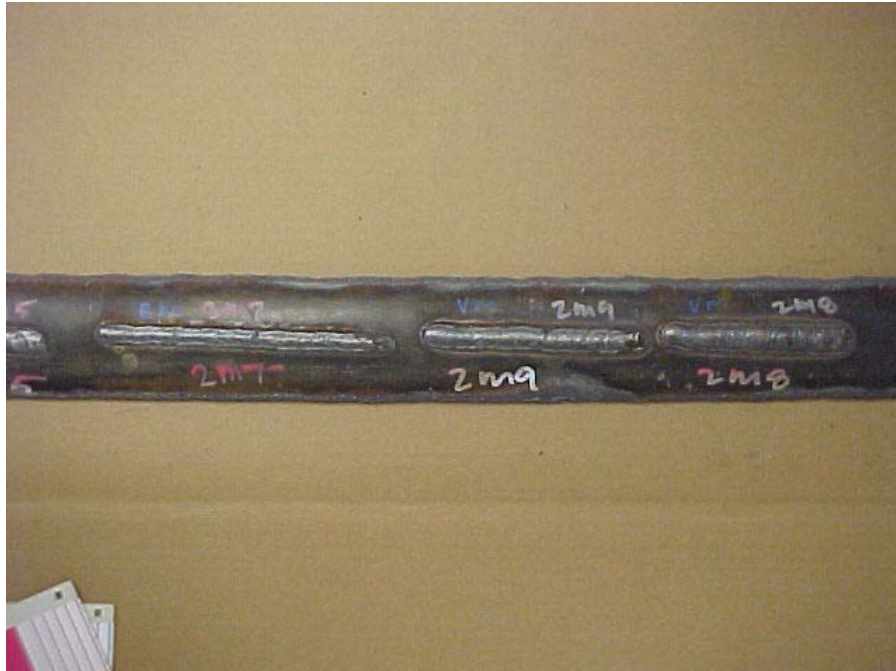
Figure 16 - External Appearance of Welds Made on 3.2 mm (0.125 in.) Thick Pipe with Methane Gas at 4.5 mPa (650 psi) and 6.1 m/sec (19.9 ft/sec) Flow Rate
