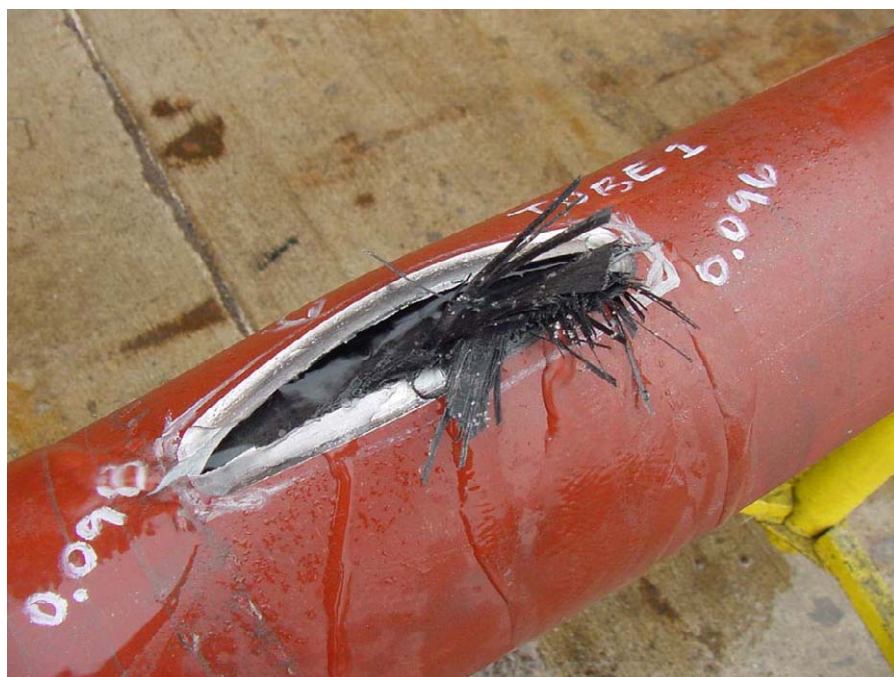
Figure 21 - Hydrostatic Test Rupture of Long, Shallow Simulated Corrosion Damage in Pipe Section Containing Fiber-Reinforced Composite Liner
