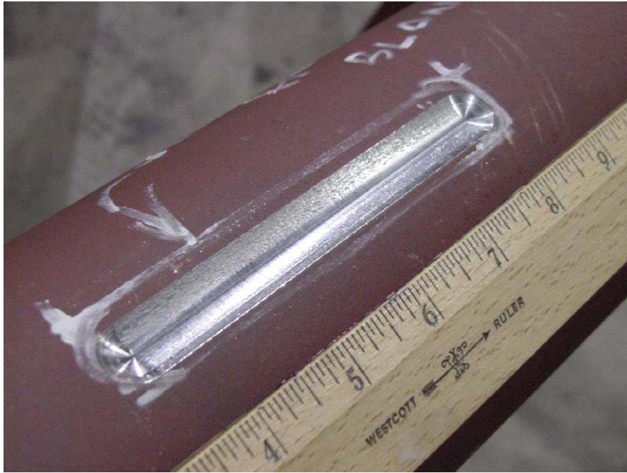
Figure 12 - Long, Shallow Simulated Corrosion Damage
