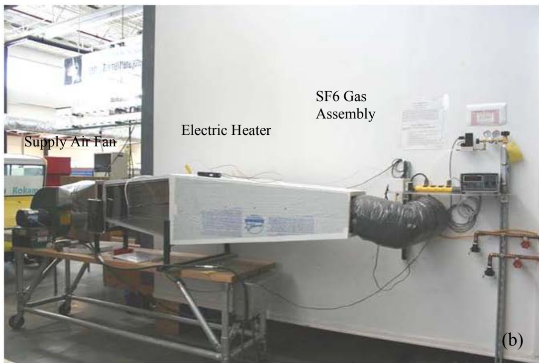
Figure 3. Schematic (a) and Photo (b) of Supply Air Apparatus – Not To Scale
