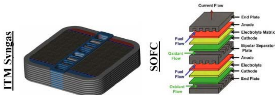
Fig. 4. Examples of fine-scale ceramic architectures fabricated by the Ceramatec process. Laminated ion transport membrane (left) and laminated ceramic solid oxide fuel cell structure (right). [Images provided by M. Ferber, Ceramatec, Salt Lake City, UT].
