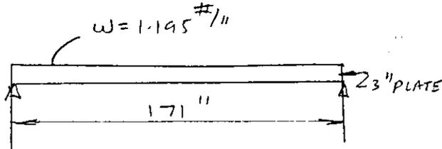
ASSUMPTION: ① DUE TO SEVERAL CUTOUT IN THE PLATE, USE DIAGONAL STRIP FOR SPAN
