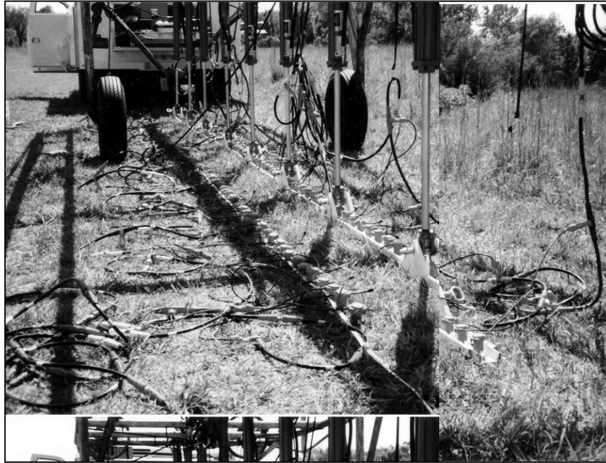
Fig.1. Automatic geophone-planting device set up for CMP data acquisition. The control line is on the left, the test line on the right. (Spikes, 2002).
