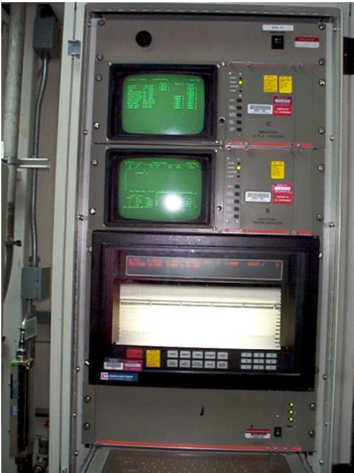
Figure 3.4. EG&G-Berthold Alpha-Beta and Tritium Monitor Display and Recorder Units
