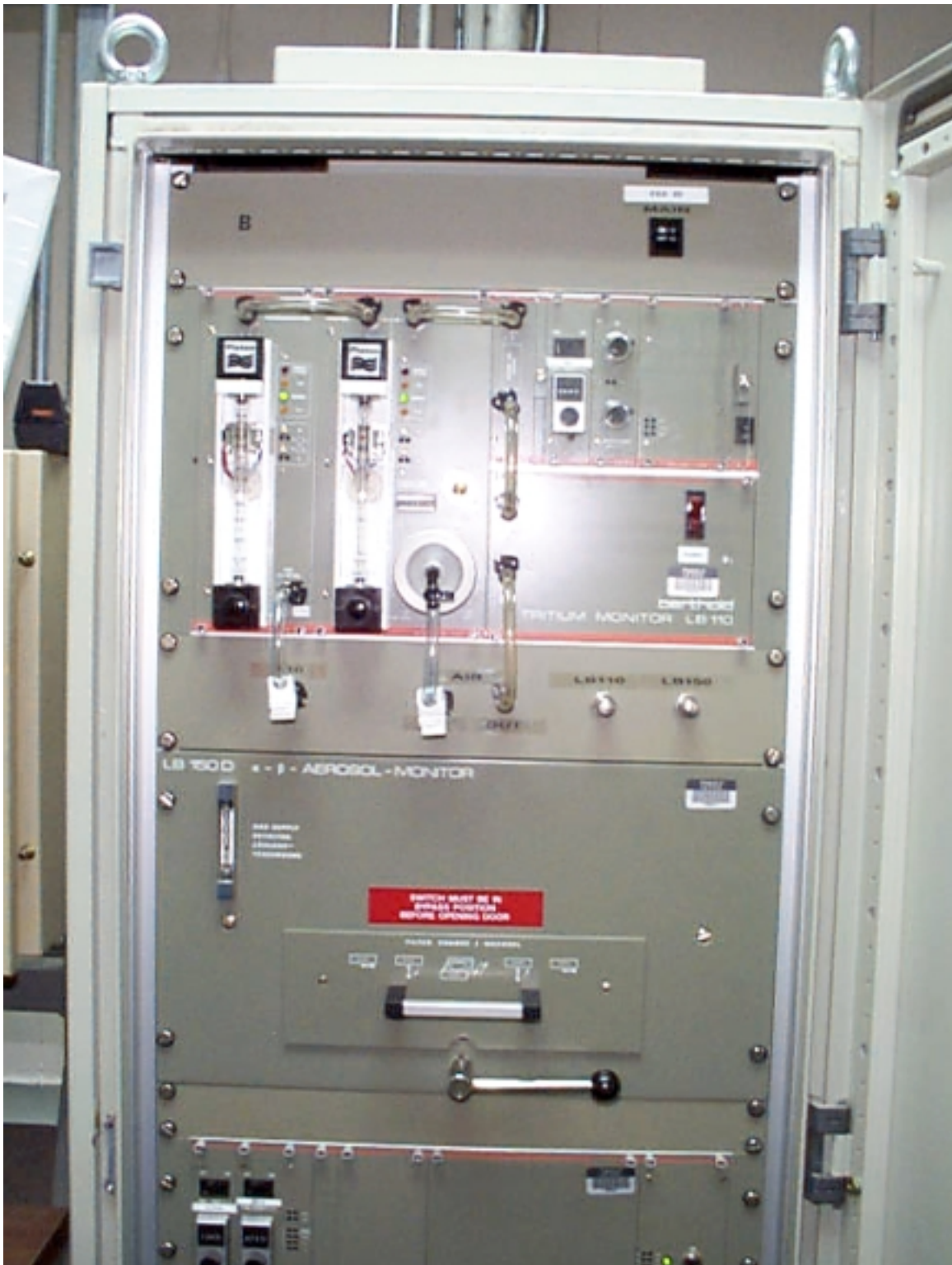
Figure 3.3. EG&G-Berthold Alpha-Beta and Tritium Monitor Detector Units
