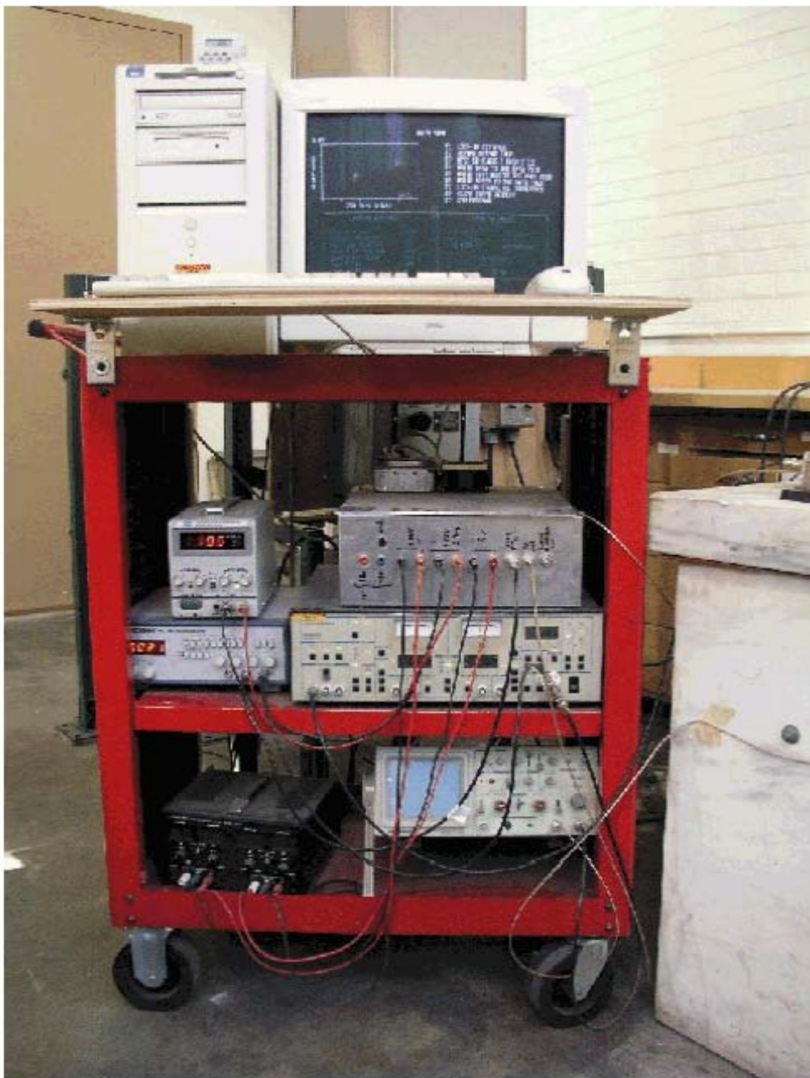
Figure 3. Data acquisition cart showing DC power supply, function generator, lock-in amplifier, and other supporting equipment for generation and control of the microwaves used by the fly ash monitor.
