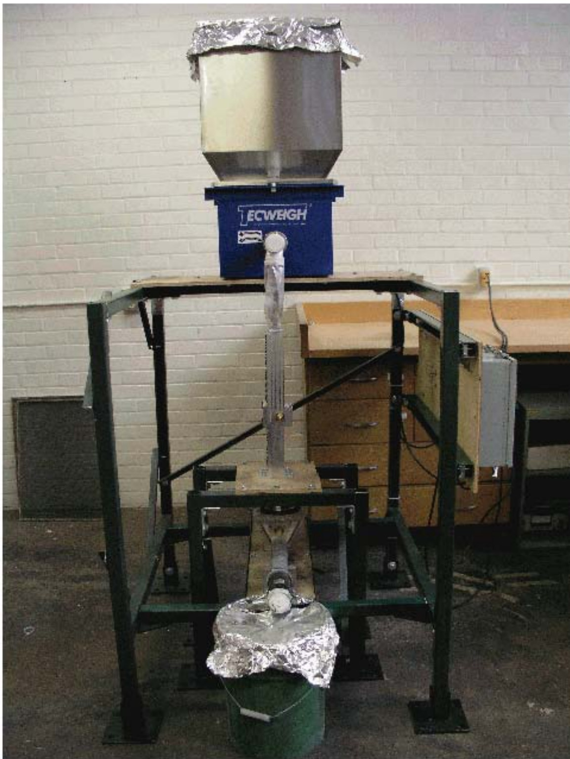
Figure 4. On-line fly ash monitor and supporting equipment.
