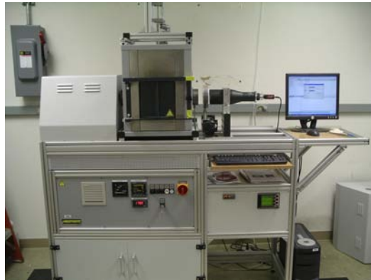
Figure 5. A photo of the Thermo Optical Mechanical Measuring Instrument (TOMMI) that was used to measure viscosity of glasses and composites at elevated temperatures.
