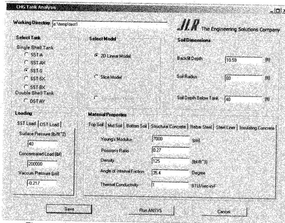
Figure 4. Run ANSYS button is lit after saving parameters
