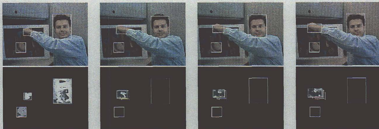
Fig. 3. Tracking of skin-color regions (top row) and depth computation (bottom row) for zoom gesture (hand moving towards the camera).
