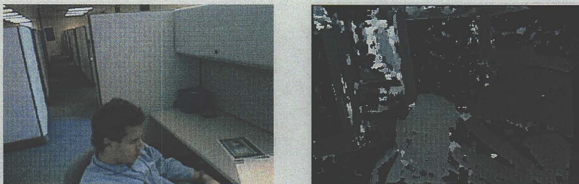
Fig. 2. Typical color and depth images produced by the stereo vision system.
