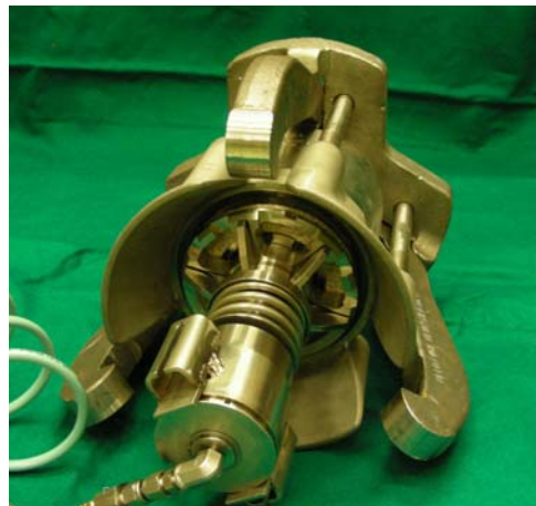
Figure 9. Installation Tool in Hanford Connector
