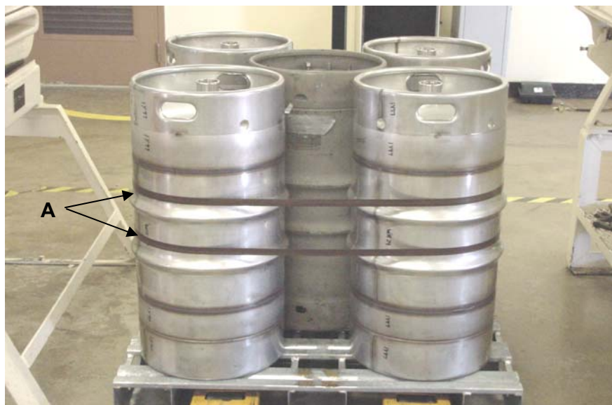
Figure 5. Digital photo of five SAFKEG drums on a galvanized steel pallet. Note strapping (A) securing drums to pallet. Pallet size is 4 feet by 4 feet. Drums will be stored 3 pallets high.
