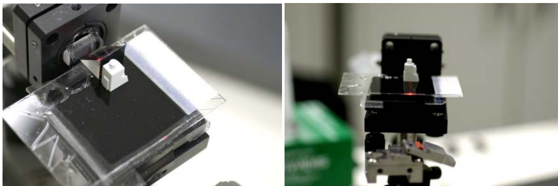
Figure 18 Experimental setup and example of light guided by sensor film: a 50 micron thick film is coated on a low index glass substrate. The index of the film is higher than the substrate, hence the film acts as a waveguide. Visible light (633nm) is directed into the waveguide using an optical fiber and a prism. The optical fiber carries the light from the source, and the prism couples the light from the fiber into the film. A small non-transparent piece of plastic was placed in front of the prism to block scattered light so that a picture could be taken. The near field view of the endface, opposite the prism, shows the light coupling out of the film. The film guides the light in a forward manner, with beam expansion only within the film.
